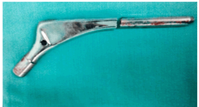
Figure 6: Detail of the fractured implant.
